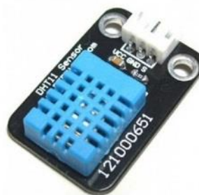
Рис. 1.15. DHT11 Temperature Humidity Sensor
